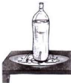
Liquid exerts equal pressure at the same depth.
